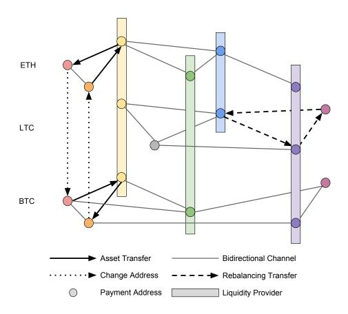
Fig. 1. Cross-Chain Atomic Swaps and Channel Rebalancing
